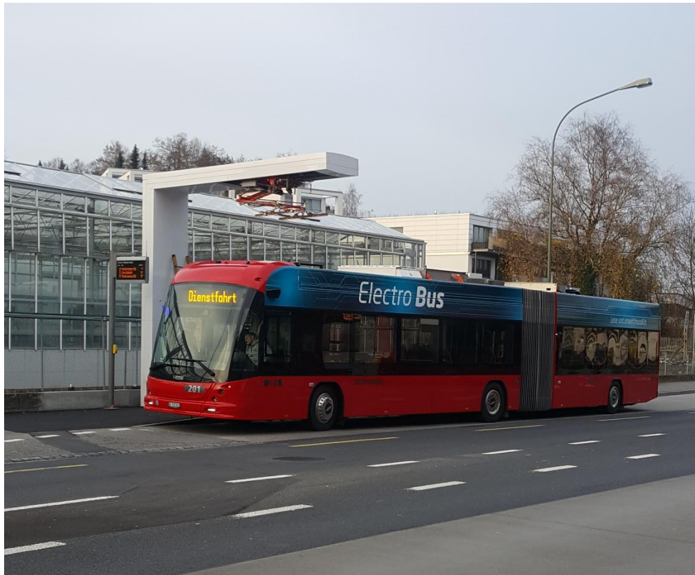
Schnell - Ladestation Electro Bus
